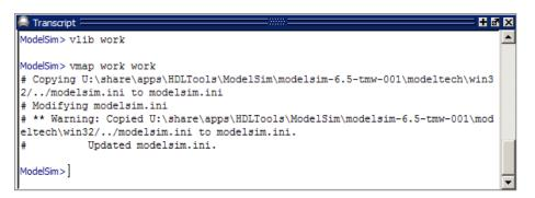
**Note** You must use the ModelSim **File** menu or vlib command to create the library folder to ensure that the required \_info file is created. Do not create the library with operating system commands.
